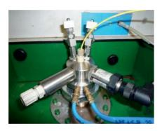
Fast microwave-enhanced reactions were monitored online by UV/Vis spectroscopy with a sensor in solution. This method is superior to slower methods (e.g. NMR, HPLC, TLC), because it is much faster and can also be performed in concentrated solutions.
